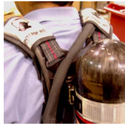
Hose cover 99154-01 installed
